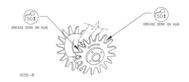
IMPORTANT: The recommended service intervals are based on normal conditions; severe or unusual conditions may require more frequent lubrication.
