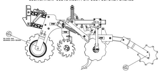
To ensure longevity and reliability of the MAVERICK OPENER™ HR Plus, the recommended lubrication schedule should be followed using multi-purpose grease at intervals as indicated.
